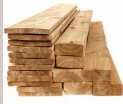
Timber used for shuttering
