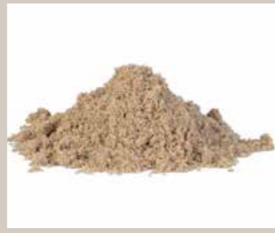
Sand used in concrete mixing
