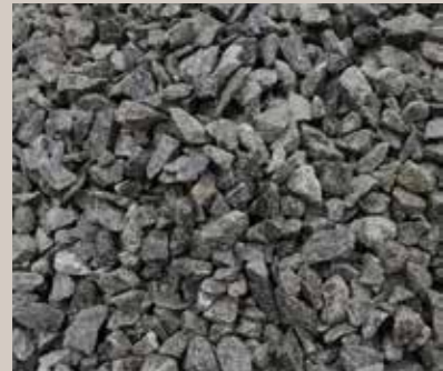
Aggregate used in concrete mixing
